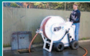
Self propelled skid-steer easement reel for restricted access and environmentally sensitive areas.
