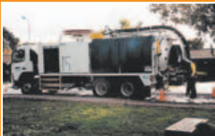
Combination Jet-Vac drain and pit cleaning and vacuum recovery.
