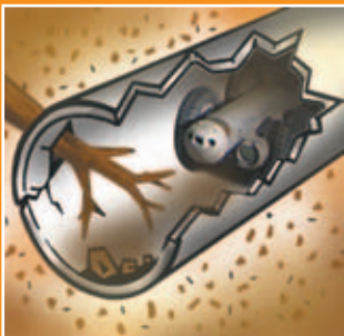
Pipeline cleaning, viewing and non-excavation repairs.
