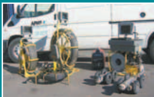
Full range of CCTV Robotic and push-through camera survey equipment.
