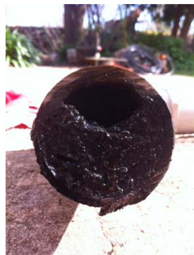
Right: Fat and grease blocking waste trap
