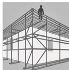
Scaffold, fully decked with hand, knee and toe rails
