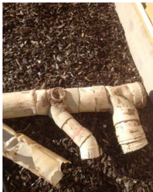
Above: Drains irreparably damaged by chemicals
